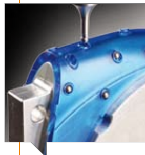
Intermediate assembly step with precision-pressing of stainless steel balls into the semi-finished product. The next step is the overmol- ding of the balls.
